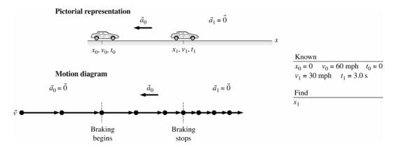
**1.37. Model:** Represent the wad as a particle for the motion diagram. **Visualize:**
